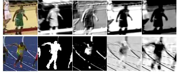
Fig. 1: Visualization of the convolutional features extracted from the first convolutional layer of AdaCFNet. Activations are shown for two sample patches (left), taken from the Basketball (top row) and Bolt (bottom row) sequence respectively. These convolutional features have different activations on the target object.
